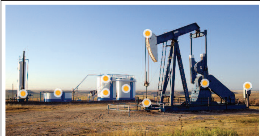
Fully integrating workflow management with remote monitoring and control capabilities allows operators to realize significant economic, operational, environmental, regulatory compliance and safety benefits with automation technology. As shown here, a variety of equipment and processes can be automated on any production site, ranging from pump controllers and tank battery levels, to ambient air quality monitors and compressor operations.
